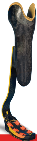
A blade or sport prosthesis — made of durable carbon fiber for high-impact activities like running, jumping and playing sports. Blades are shaped like a "C" or "J," compress under body weight and help amputee athletes rebound quicker and use less energy.
