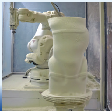
Orthotics and Prosthetics Technical Supervisor Bob Rowan, C.T.O., creates a customized scoliosis brace using the 7-axis Vorum carver, a generous gift funded by John Martinson.
