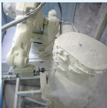
Orthotics and Prosthetics Technical Supervisor Bob Rowan, C.T.O., creates a customized scoliosis brace using the 7-axis Vorum carver, a generous gift funded by John Martinson.
